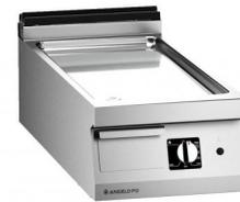
Griddle made of AISI 304 stainless steel, 20/10 mm thickness top. Cooking plate made in Fe510D steel with hard chromium surface treatment. Delivered with: plate plug. Heating by burner group controlled by modulating thermostat valve, safety thermostat. Working temperature (min-max): 100-280°C.
